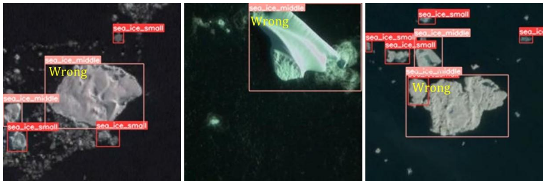
(c) YOLOv8 incorrectly predicts large-scale sea ice as medium-scale sea ice.
