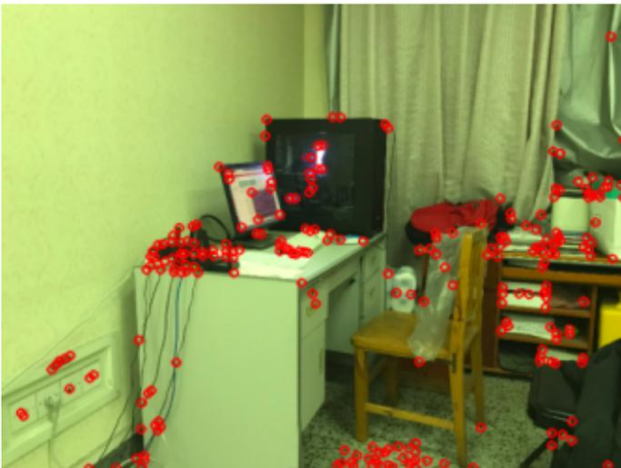
Figure 4. Image of extracting feature points without mask
