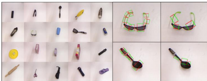
Figure 1. The Cornell Grasp Detection Dataset contains a diverse array of objects, each labeled with multiple graspable and ungraspable feature labels.
