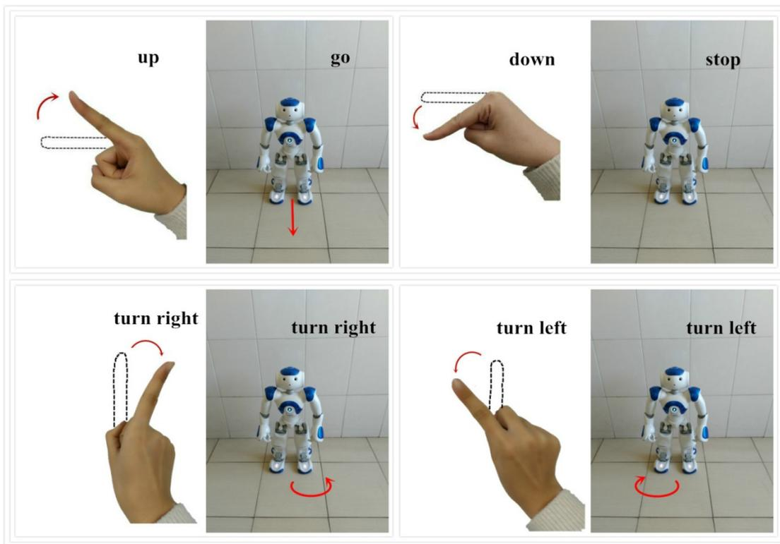
Figure 5. The relation of gesture and robot movement.
