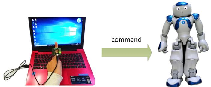
Figure 3. The finger attached to the inertial transducer.
