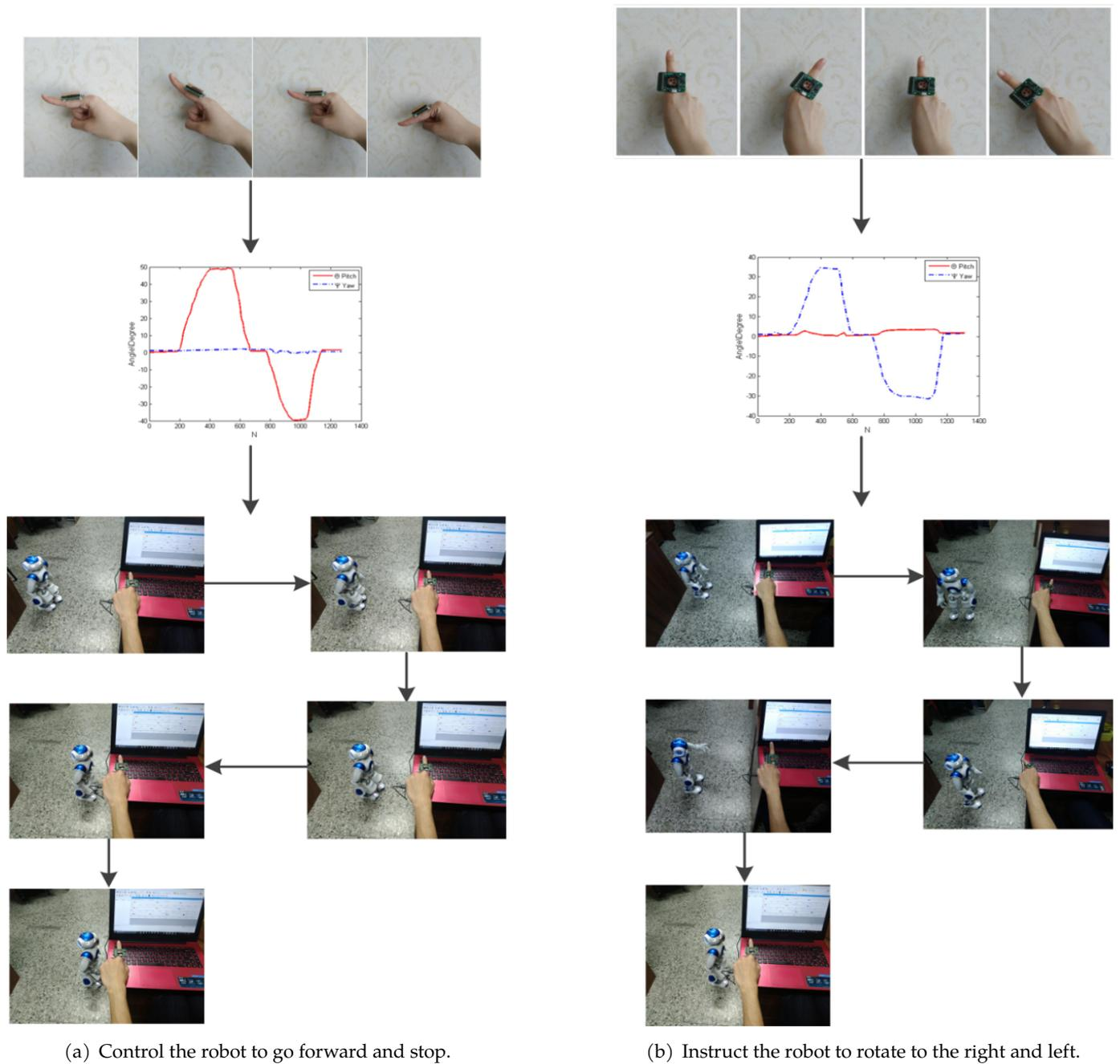
Figure 10. The finger gestures and robot movements.
